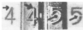
FIG. 3 — The reproduction of two damaged typefaces and the corresponding imprints from these numerals. The flattened area at the top of the 4 is not easily discerned on the imprint on the delivery slip but with experience can be recognized by the slight widening of the pointed top.
